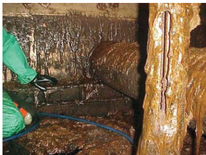
Fig. 1 Naphthenate deposits in crude oil processing equipment, by courtesy of Oil Plus Ltd., UK.
